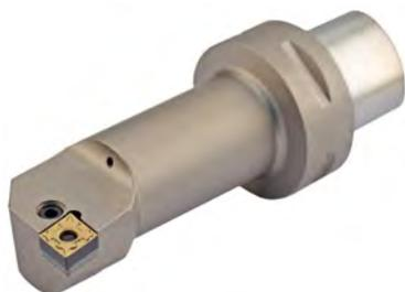
Characteristics: Boring bar for internal turning applications equipped with rhombic negative inserts (angle 80°). PSC with internal coolant.
