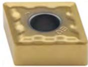
First recommendation for medium cutting of stainless and mild steel and for light cutting of difficult-to-cut materials. Double-sided chipbreaker. The sharp cutting edge gives best performance.
